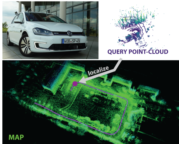
Fig. 1: We aim at accurately localizing our vehicle in a map build from previously collected LiDAR point clouds. A query point cloud scan is fed through the OREOS pipeline, yielding a compact descriptor that allows to retrieve near-by place candidates from the map, and estimate the yaw angle discrepancy. With this information, a local registration method, such as ICP, can be bootstrapped and used for subsequent high accuracy localization along the traversal.
